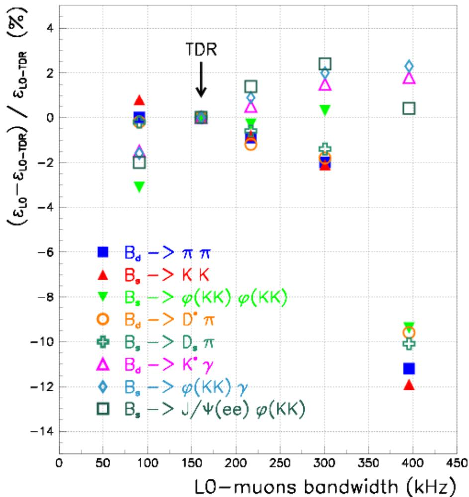
\* losses less than 4% up to 300 kHz
